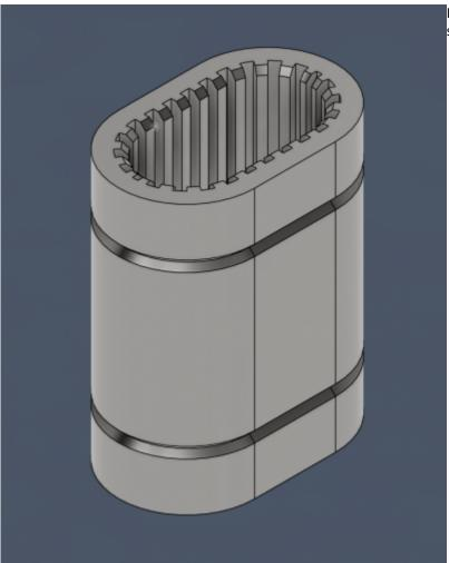
I created some oval shaped linear bearings for starters and testing them on the rails.
