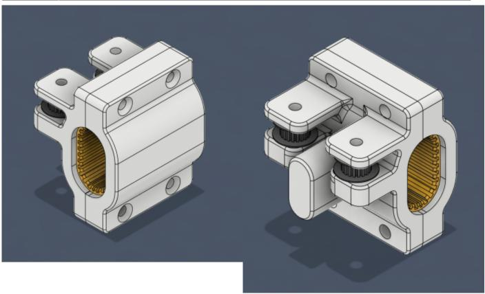
Then created some bearing holders with idler pulley holders and mounts for the cross bar.
