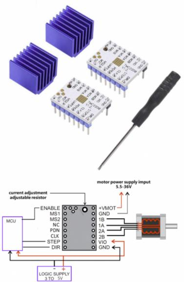
So some further research had some reasonably costed silent steppers and I opted for some TMC2208<sup>14)</sup> drivers from Amazon and tested then out. I got two for around €9.00, and wired up a motor to a pico 2040 and proceeded to do some tests.
