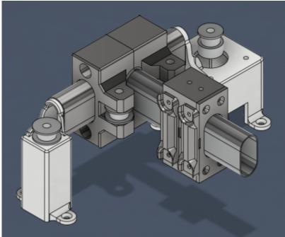
The final design for the core-xy linear stage is here: https://www.printables.com/model/1143004-budge t-core-xy-linear-rail-system. The print layout file includes a mirrored layout of the left stage stepper and idler holders.
