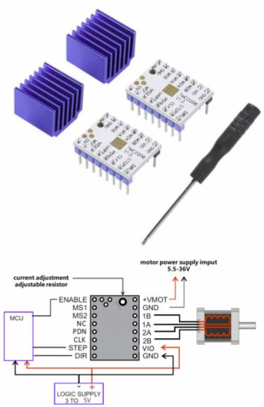
So some further research had some reasonably costed silent steppers and I opted for some TMC2208 drivers from Amazon and tested then out. I got two for around €9.00, and wired up a motor to a pico 2040 and proceeded to do some tests.
