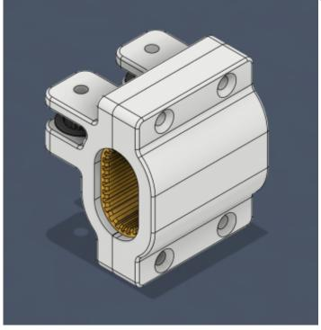
The cross bar fit was also tight and I used a mallet to drive it on to avoid play. I realised I did not fit the bearing and designed a split bearing.
