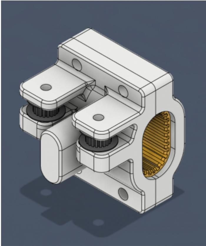
Then created some bearing holders with idler pulley holders and mounts for the cross bar.
