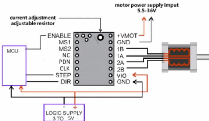
So some further research had some reasonably costed silent steppers and I opted for some TMC2208 drivers from Amazon and tested them out. I got two for around €9.00, and wired up a motor to a pico 2040 and proceeded to do some tests.
