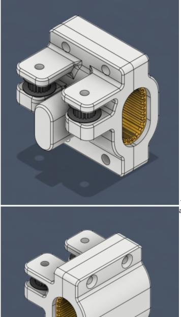
Then created some bearing holders with idler pulley holders and mounts for the cross bar.
