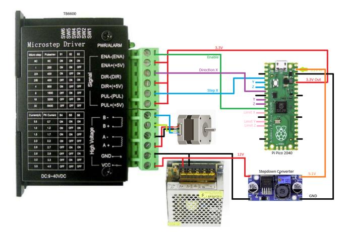
This schematic show the wiring for the X axis, the two Y axis connections for direction and step should be used instead.
