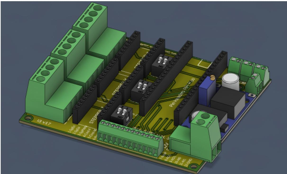
The final design include PCB headers for the pico and all the drives with pluggable terminal connectors for the motors and screw terminals for expansions. The board also includes an adjustable step down regulator for 5v power for the Pico.
