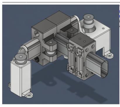
The final design for the core-xy linear stage is here: https://www.printables.com/model/1143004-budge t-core-xy-linear-rail-system. The print layout file includes a mirrored layout of the left stage stepper and idler holders.
