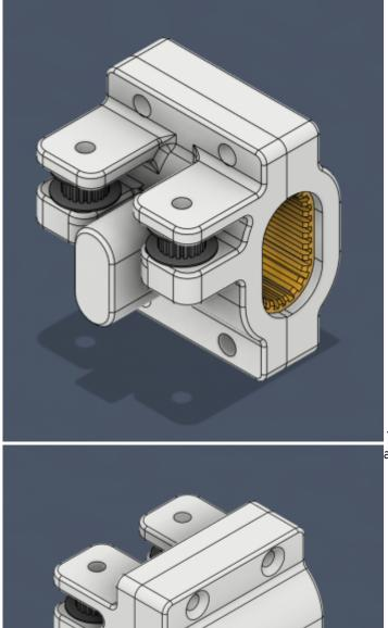
Then created some bearing holders with idler pulley holders and mounts for the cross bar.
