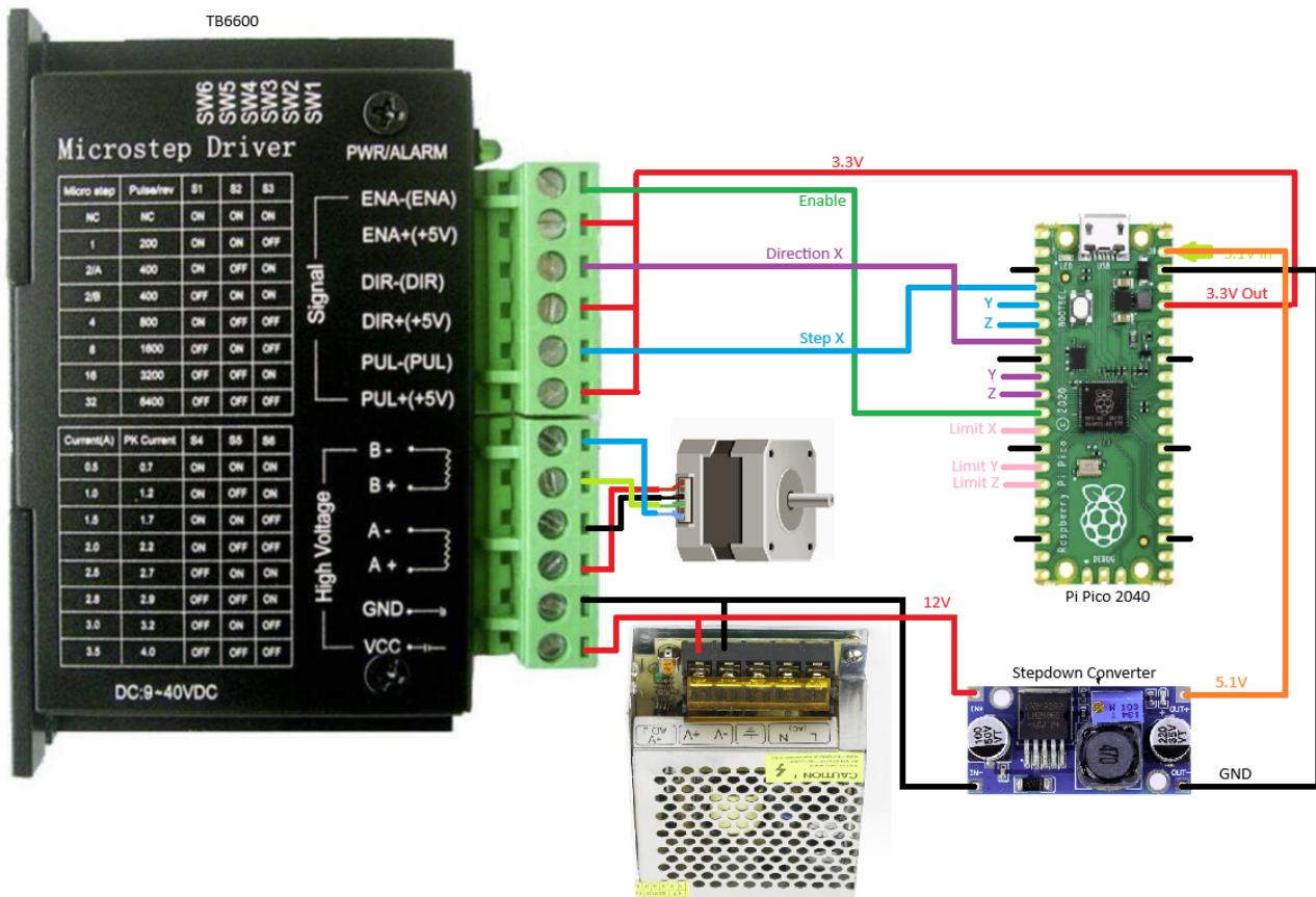
This schematic shows the wiring for the X axis, the two Y axis connections for direction and step should be used instead.
