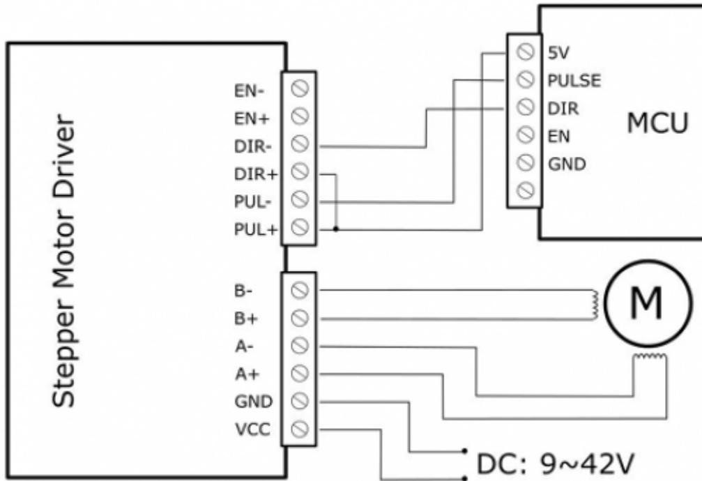
So in keeping with the proposed vendor Microcontroller wiring we then add the enable lines back in and it should look like this.
