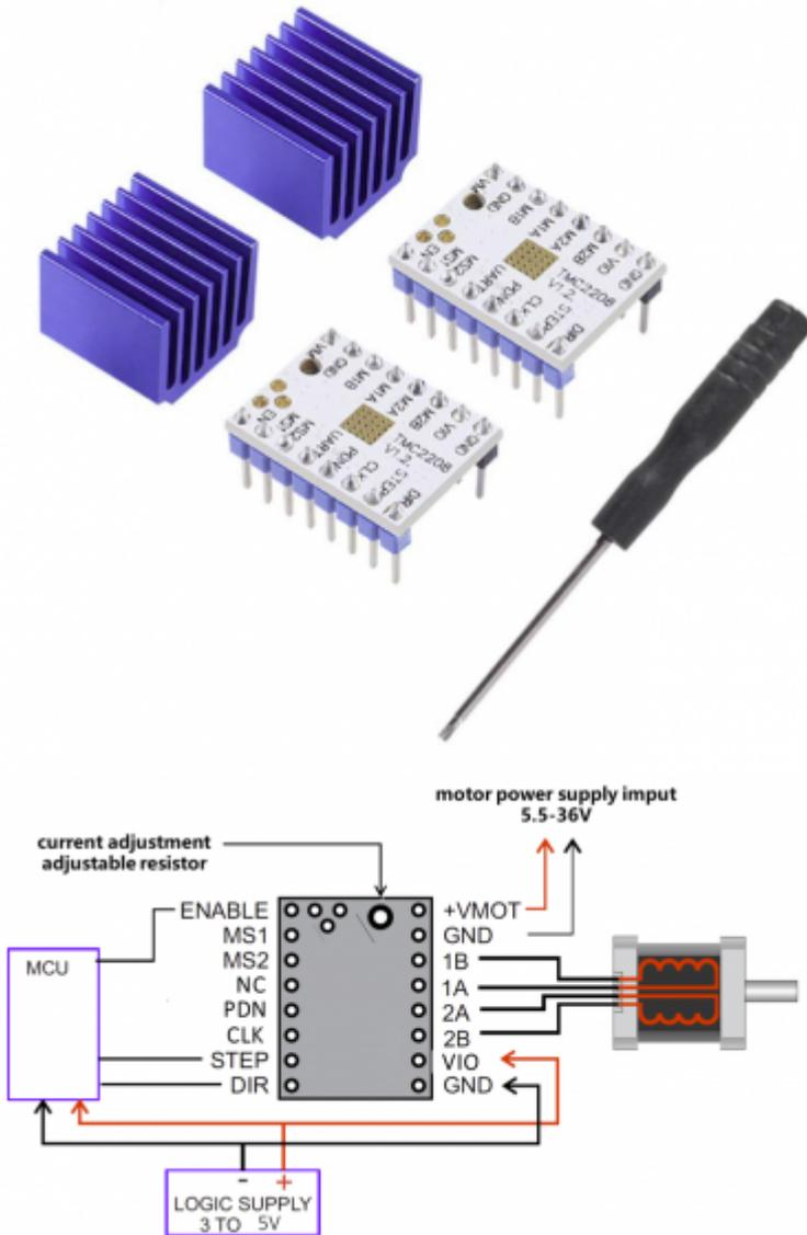
So some further research had some reasonably costed silent steppers and I opted for some TMC2208<sup>14)</sup> drivers from Amazon and tested them out. I got two for around €9.00, and wired up a motor to a pico 2040 and proceeded to do some tests.
