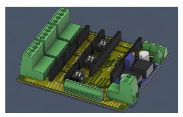
The final design include PCB headers for the pico and all the drives with pluggable terminal connectors for the motors and screw terminals for expansions. The board also includes an adjustable step down regulator for 5v power for the Pico.
