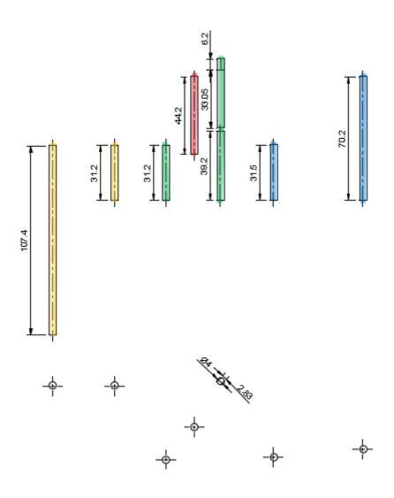
The bearings selected for this project has a 4mm inner diameter, so the shafts to be prepared is 4mm thick and of various lengths as show in the diagram above.
