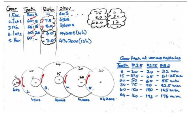
Combining whiteboard designs and sketching using fusion I managed to figure out a layout and some ratios that can work.
