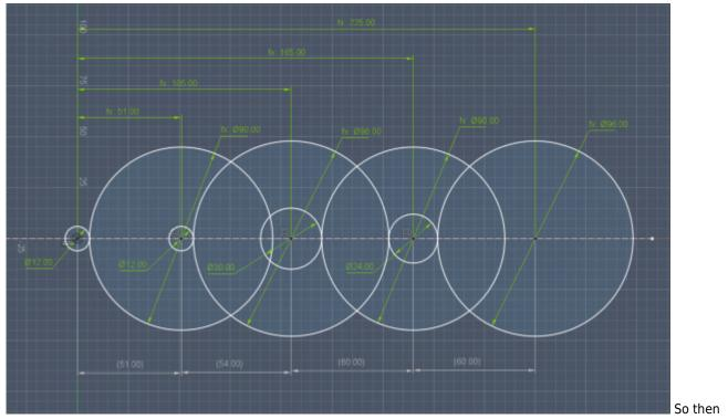
working backwards with the gear pitch<sup>5)</sup>, through trail and error I managed to get to this solution in a straight line.
