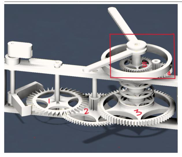
So using the same numbers for the gears in the table above, you can see the same gearing pattern in the bottom layer, but the hour hand gears are on the minute shaft. I have seen this on exploded views, but not in a layout like above that made sense. So the final iteration will attempt to incorporate this idea, back to the drawing board....
