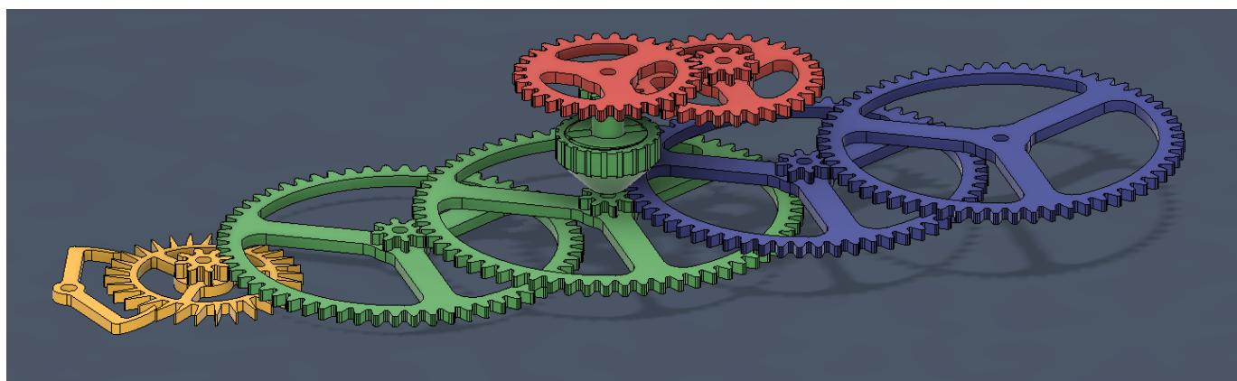
So this is a coloured view of the entire drive train with the yellow parts being responsible for generating the seconds, green then stepping that down to minutes and delivering the output to a shaft driving the minute hand. The red gears then steps everything down further by a combined ratio of 12 and driving the hour hand. Lastly the blue gears stepping down everything by another ratio of 56.25 to provide enough power for 10 days.
