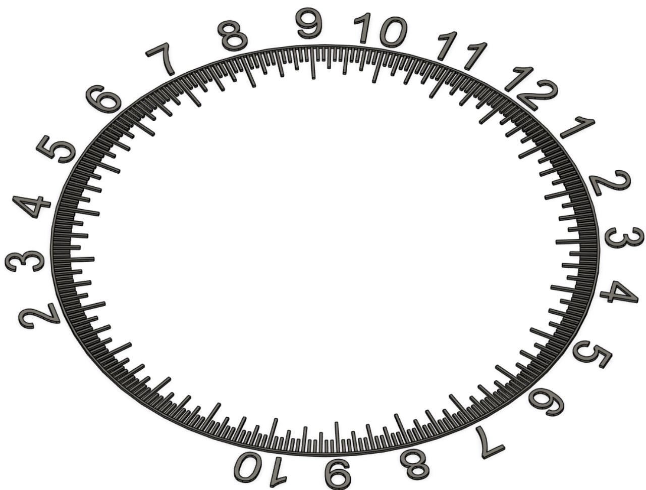
Then create the faceplate on the same layer, extruding downwards to create a thicker body that the parts in step one, for example, the numbers and lines in part one I created is 0.8mm deep, so will be four layers deep with a print height set at 0.2mm. The Faceplate body I extruded to 3mm.
