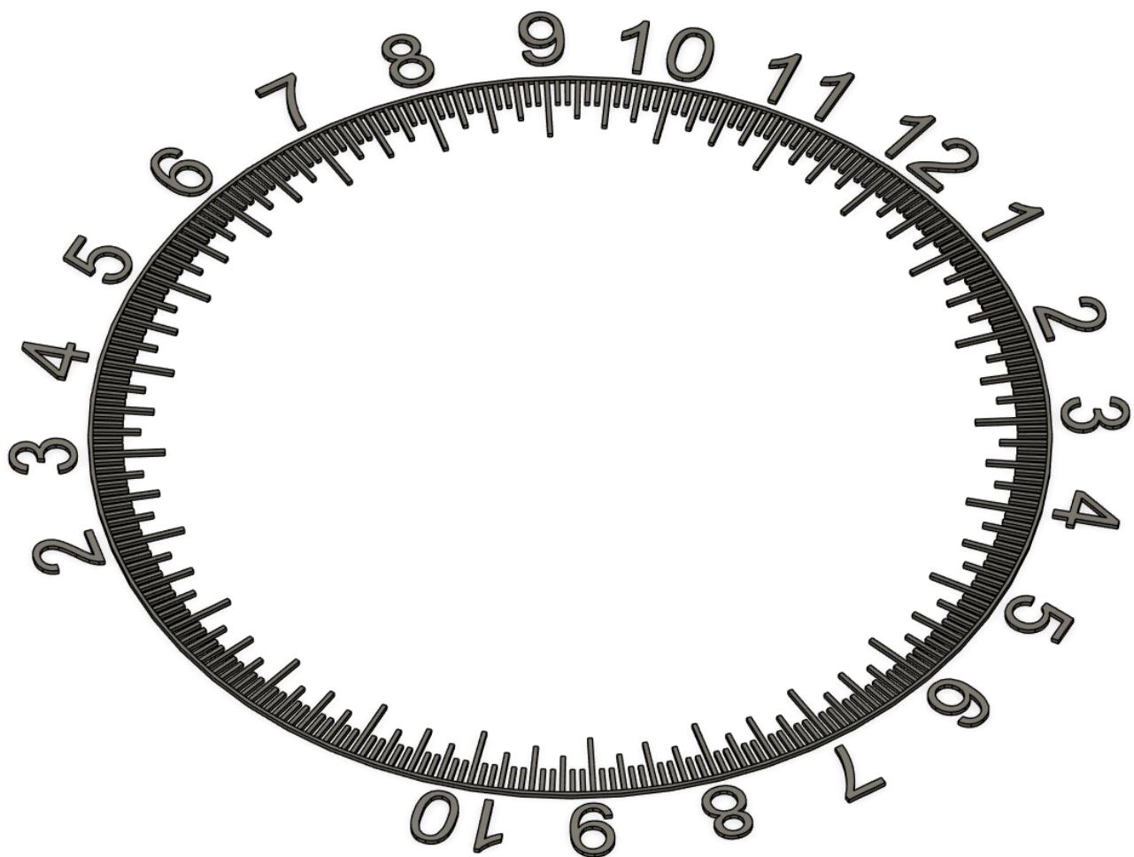
Then create the faceplate on the same layer, extruding downwards to create a thicker body than the parts in step one, for example, the numbers and lines in part one I created is 0.8mm deep, so will be four layers deep with a print height set at 0.2mm. The Faceplate body I extruded to 3mm.
